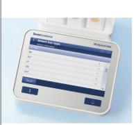
The twelve most commonly used ion types are pre-programmed in the instrument making the settings as convenient as possible. For others you can enter the ion charge and molar mass to ensure that all calculations and conversions are done for you.
